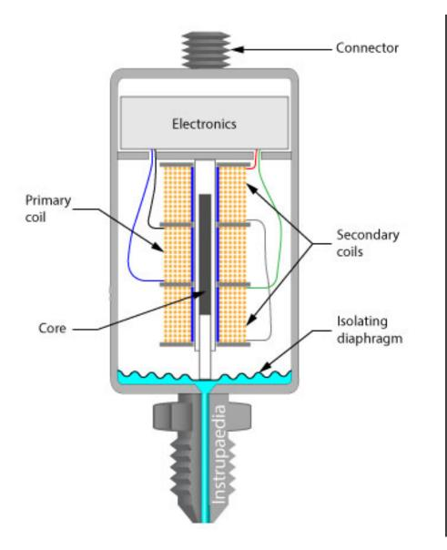
Inductive – a post moved by pressure changes induces a current between coils in a transducer
