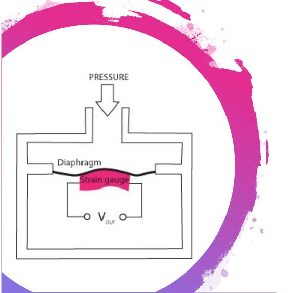
Strain gauge – uses strain gauges to measure membrane deflection via piezoresistance Variable reluctance – change in diaphragm deflection causes magnetic reluctance in circuit
